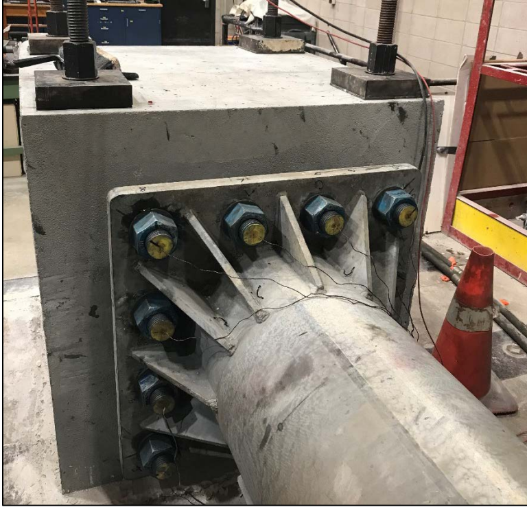
Figure 3.36 - Concrete Block Following Post-tensioning
