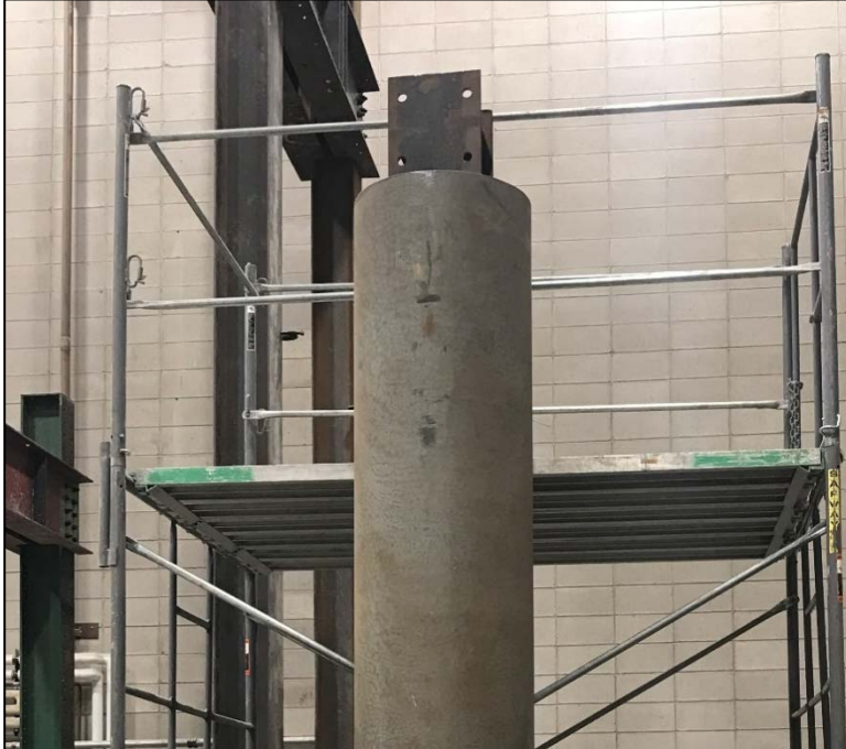
Figure 3.33 - H-Pile Placed Inside Sign Post
