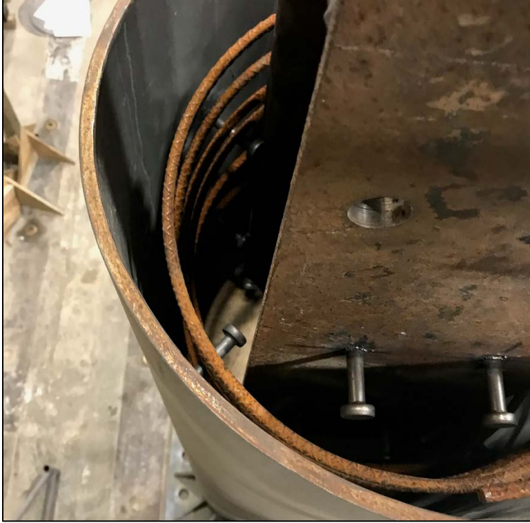
Figure 3.32 - HP10x57 and Confinement Placed in Sign Post
