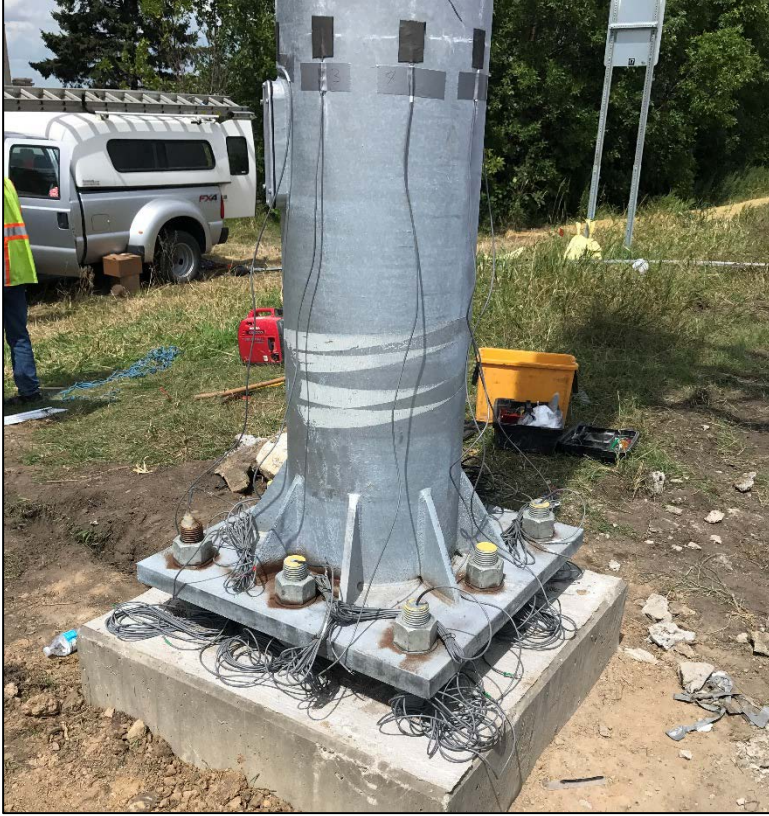
Figure 3.8 - Anchor Bolt and Post Strain Gages
