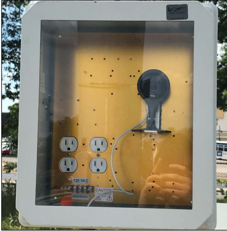
Figure 3.12 - Camera Inside Enclosure
