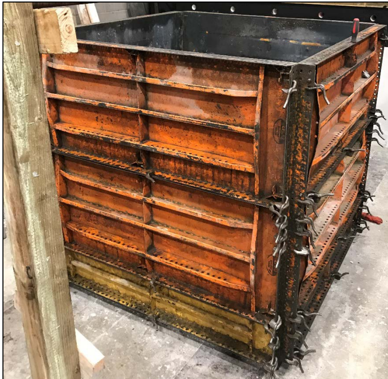
Figure 3.25 - Concrete Block Formwork
