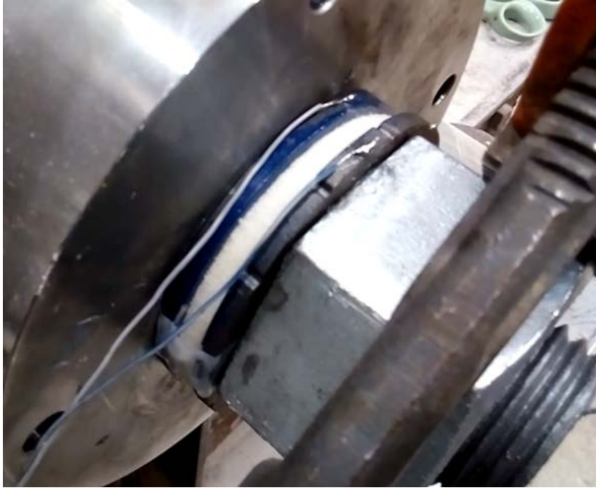
Figure 6.5 - Memory Foam Capacitor during Loading
