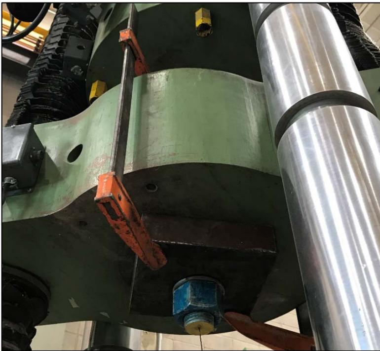
Figure 3.7 - Calibration of Anchor Bolts
